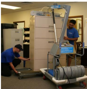
Specialized Equipment Boxless Move with Spider-Crane
